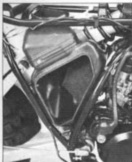
Plastic airbox has an extended top to keep water out. Removal of the oiled foam filter is simple and doesn't require tools; pulling the rubber strap and removing the cover gives access.
