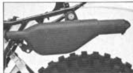
Spark arrester/silencer is forestry legal and best of all, it's super quiet.
