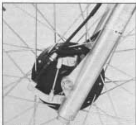
Double leading shoe front brake is the same as the YZ's except it's less grabby. Brake cable has a heavy outside sheath to prevent flexing, housing is integral with the adjuster so the housing can't jump out.
